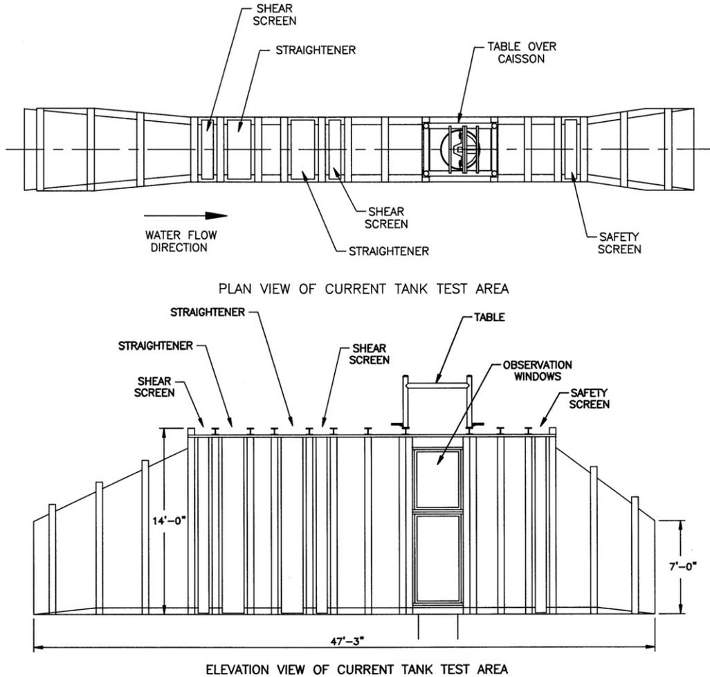
Fig. 1. Current tank test area plan and elevation view (1 ft = 0.3048 m).
