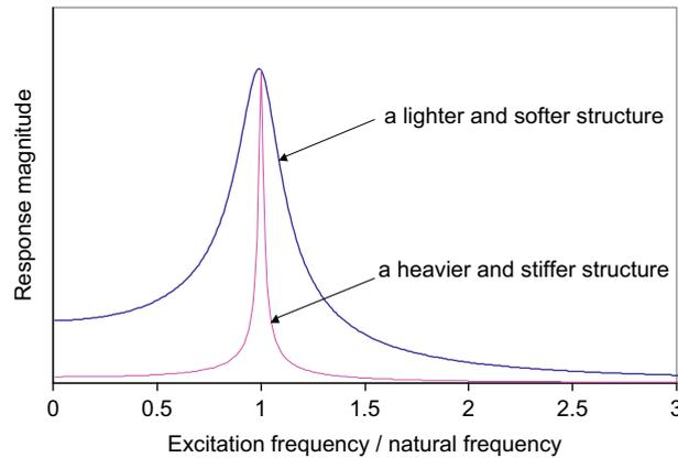
Fig. 8. Response bandwidth of a lighter/softer structure and a heavier/stiffer structure.
