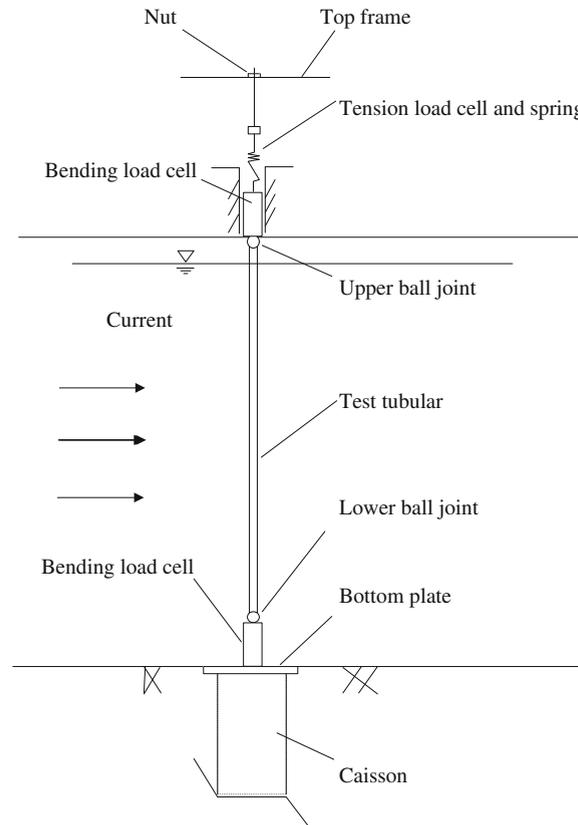
Fig. 2. Test set-up.
