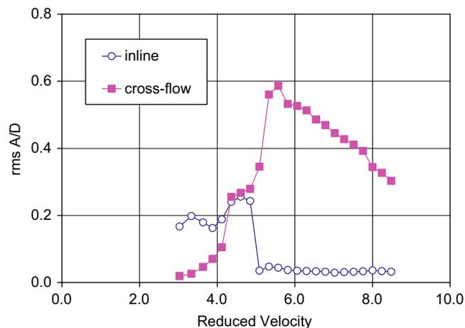
Fig. 6. VIV motion magnitudes of the 4.5 in cylinder.
