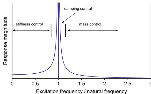
Fig. 7. Stiffness, mass, and damping controlled zones of a resonator.
